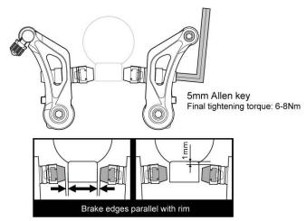
(3) Thread the brake cable though the center bolt on the straddle cable carrier making sure that there is a minimum of 20mm between the end of the cable housing and the top of the straddle cable carrier. Hold the straddle cable carrier center bolt with a 5mm Allen key and tighten the nut using a 10mm spanner.
