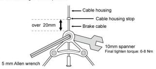
(4) Slip the straddle cable into the barrel adjuster, through straddle cable carrier and then the under the anchor bolt plate. Pull the cable tight until the brake pads contact the rim. Using a 5mm Allen key tighten the anchor bolt to a torque of 6-8mm.
